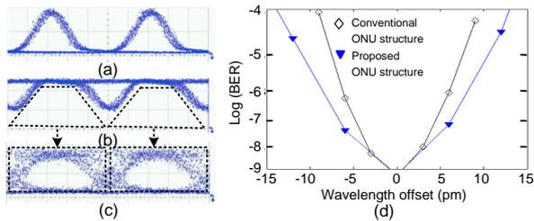
Fig. 2. Eye diagrams of (a) the demodulated downstream 10-Gb/s DPSK signal from the destructive port of the 0.25-bit DI, (b) IRZ-shaped output from the constructive port of the 0.25-bit DI, (c) the detected upstream OOK signal. Time scale: 20 ps/div. (d) BER degradation (from  $10^{-9}$ ) caused by wavelength offset between the laser source and the DI.
