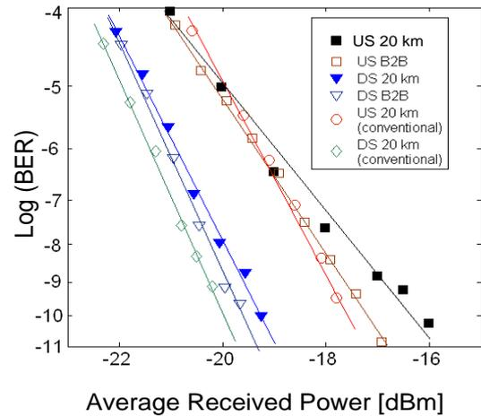
Fig. 3. BER measurement results for both down- and up-stream signals.
