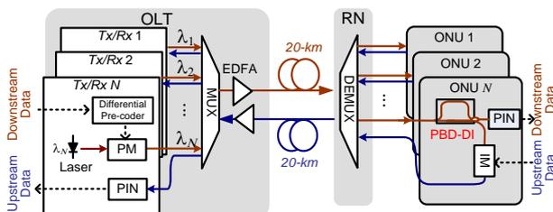
Fig. 1. WDM-PON architecture using the proposed simplified ONU structure with partial-bit-delay DI (PBD-DI).
